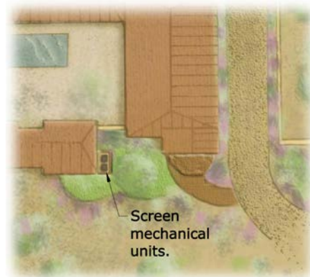
Screening Mechanical Units
