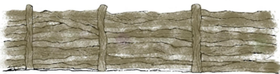
③ Indigenous Wood Corral Fencing - Horizontal Horizontal posts stacked between vertical posts
